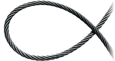
**1. The start:** A rope should never be allowed to accumulate twist as shown here because it will loop and eventually form a kink. If this loop is removed before being pulled down tight, you can normally avoid the kink.
