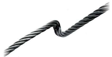
**3. The result:** Even if the wires do not appear badly damaged, the rope is still damaged and must be replaced.
